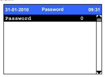
Press the Enter button to start editing mode and enter the correct password with use of the up and down arrows. Press the Enter button to select it.
