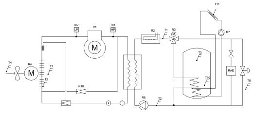
Ground source to water, no solar panel, heating tank on heating system
