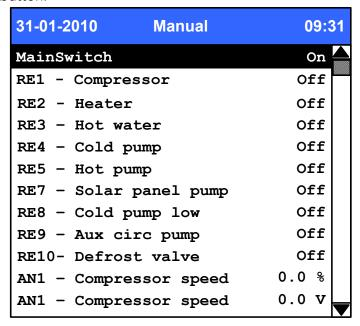
In MainSwitch field, **On** means the unit is running, **Off** the unit is stopped and **Manual** that the outputs can be operated from this menu for service purposes. Manual mode should be used by trained personnel only!
