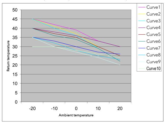
A poor insulation level means a higher impact of the ambient temperature on the room temperature and requires a higher calculated return water temperature.
