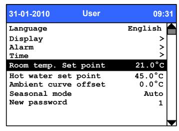
In the Ambient / Room temperature compensation menu, **Installer – Ambient / Room compensation** the level of compensation can be set.
