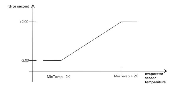
The first 5 second after start a constant preset voltage (Ustart) is sent to the inverter. After that a voltage linear to the capacity is sent to the output (see graph below). The rate of capacity change is limited to max 1% per second.
