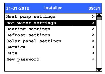
Press the Enter button to open the How water settings menu
