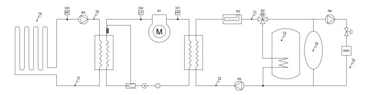
Ground source heat pump with dual condenser
